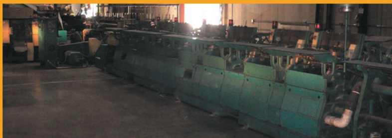
KOLBUS 16 CLAMP PERFECT BINDER WITH 3 KNIFE TRIMMER CONVEYOR AND DELIVERY • NORDSON GLUE SYSTEM
